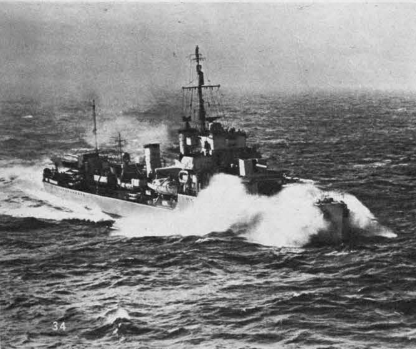
"A" AND "B" CLASS ships like Antelope (below) were first to mount their torpedo tubes in banks of four, to introduce box-shaped shields.
